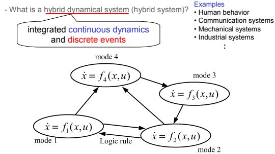
There are multiple modes and logic rules in a hybrid dynamical system.
